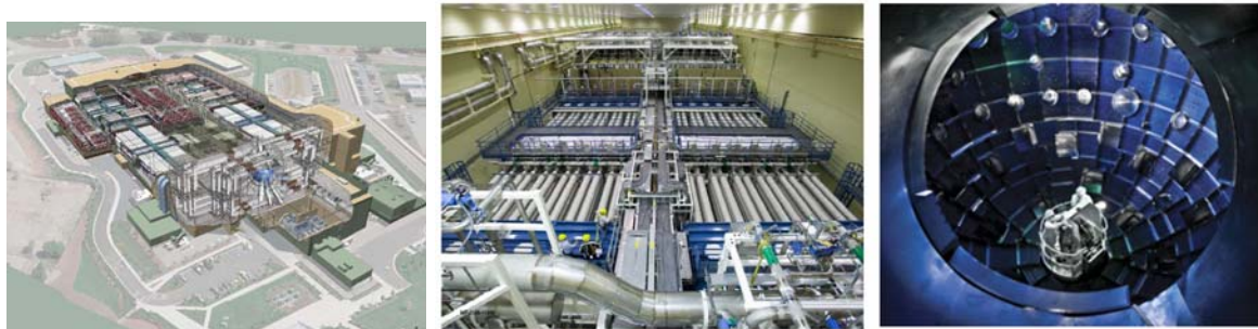
Fig. 2 NIF 1.8MJ laser system (left) & photos of laser bay (center), target chamber (right)
