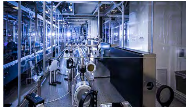
LLNL pump laser for HAPS for ELI (10 Hz, ~200 joules, ~5-10 nsec pulse)
